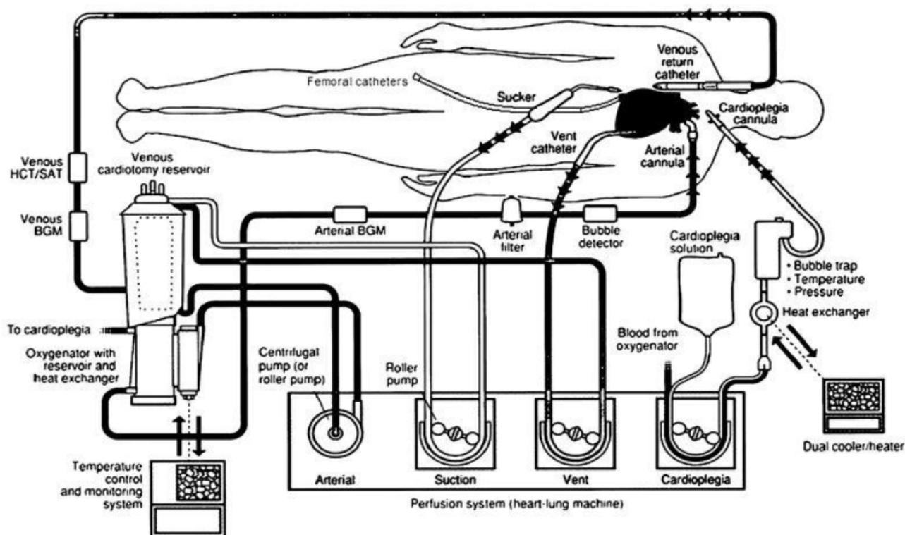
Figure 1: Typical configuration of a basic CPB circuit. BGM = blood gas monitor; SAT =oxygen saturation<sup>[9]</sup>.
